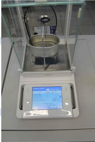
Figure 1: Density scale: First the mass of the O-ring is determined in air, then in the oval vessel filled with ethanol below.
