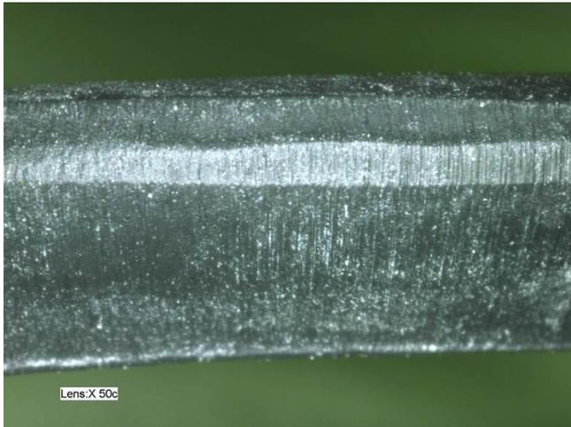
**Fig. 6:** Plan view of the outer diameter of the damaged O-ring from Fig. 5 with clear marks from the abrasion process.
