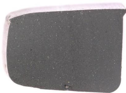
**Fig. 3:** Permanent deformation due to chemical degradation - the stronger degree of deformation in the left area can be clearly seen (medium side)
