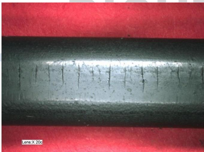
**Fig. 4:** In addition to permanent deformation, a typical impermissible thermal stress is complete embrittlement, which is shown here in crack formation after slight bending stress in the contact area of the seal.
