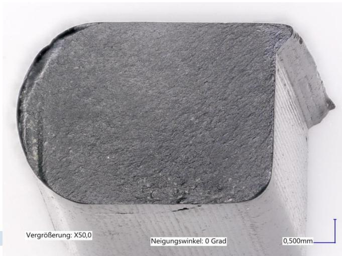
**Fig. 2:** Cross-section of a damage O-ring: In addition to the permanent deformation, a typical impermissible thermal stress is a complete embrittlement, which is indicated here in the structure of the sectional surface.
