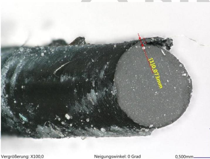
**Fig. 3:** Typical damage pattern of a gap extrusion
