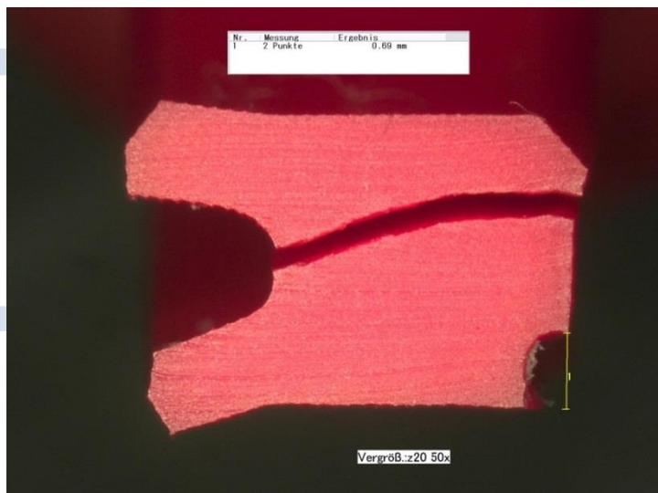
**Fig. 1:** Damage at the sealing gap of a hydraulic seal and subsequent rupture due to hydrolysis
