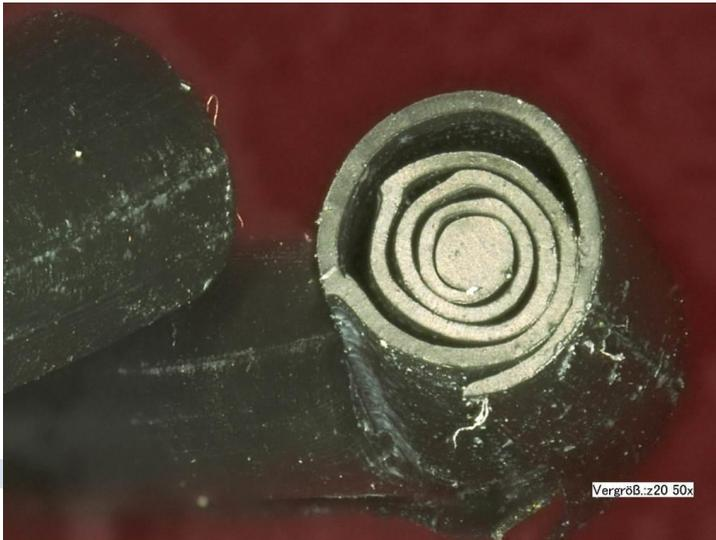
**Fig. 2:** Gap extrusion of an O-ring through sharp-edged groove recess ( $p = 350$  bar,  $gap = 0.05$  mm)
